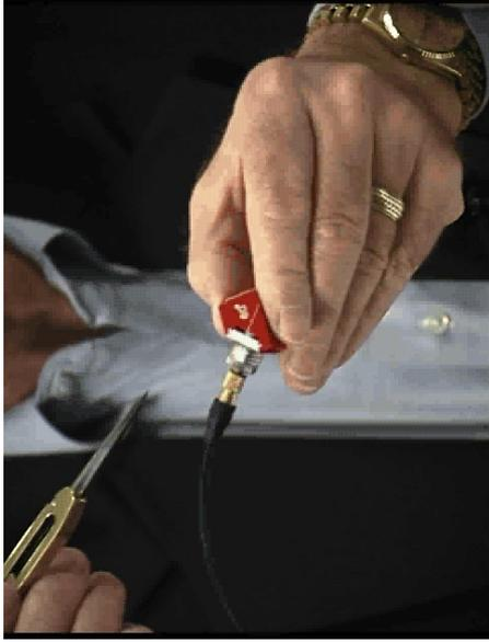
Angle beam probes are used to reach areas where normal beam inspection is either difficult or impossible. The characteristics and construction of the probe are described in this video.
