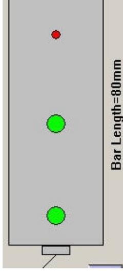
The energy burst (green sphere at the top left) travels through the material at a fixed speed. The thickness of the part is indicated by the location of the back echo. In the lower view, there are two energy spheres since one has bounced off of the bar end, and the other off of the echo flaw (red circle).
